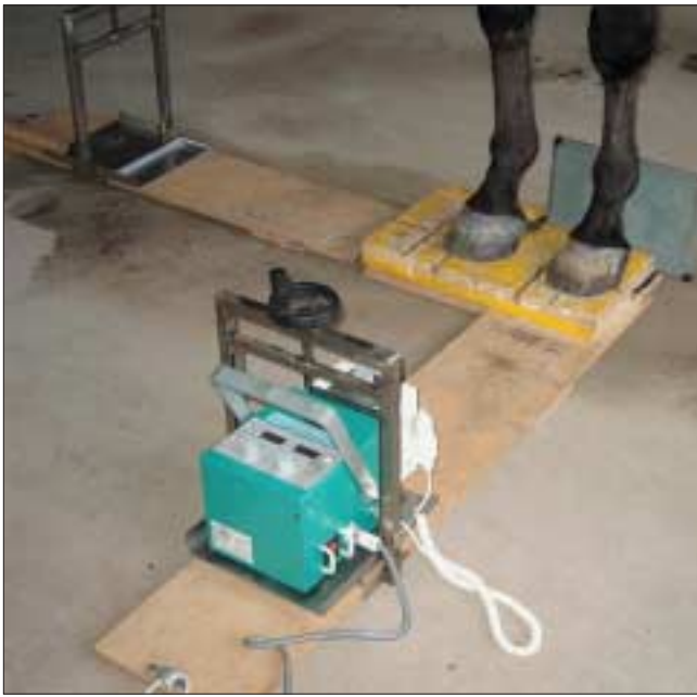
Figure 1. All radiographs were taken with the limbs positioned on a special platform, which allows taking dorsopalmar radiographs at the same level as the lateromedial.
